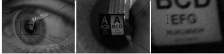
Figure 9. Image taken with a macro lens from very short distance, with realistic distance between the monitor and the eye. Readability is limited by the resolution of the camera.
