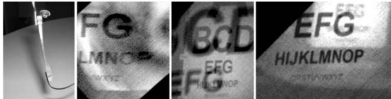
Figure 10. Reflections in two different pairs of glasses, taken from a distance of 5m. Both the inner side and the outer side of glasses produce reflections. The 18pt font is readable from the reflection.
